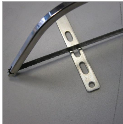
Screw to the holding device of the mounting plate. Required holes in OFL 1.0 are already pre-drilled. If necessary, the length of the magnetic holder must be altered.
