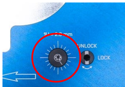
Fig. 8 Using the locking device
