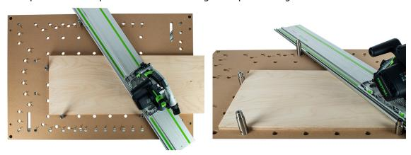
Before you cut the workpiece with the set angle, please check whether the tool, e.g. the plunge saw, can be moved over the workpiece without hitting the bench dogs. If this is not the case, adjust your set up.
