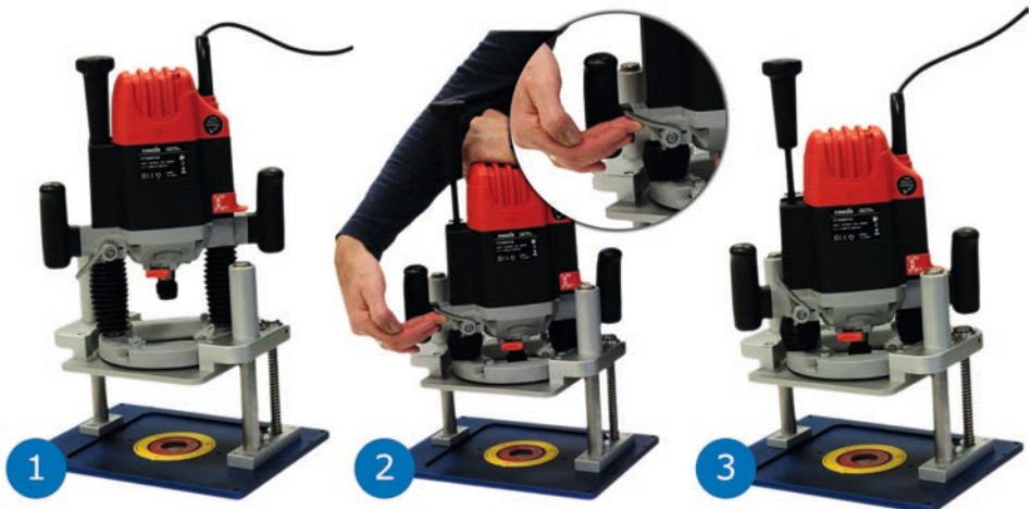
Fig. 10 Minimizing the milling height loss (OFL1.0 as example)
