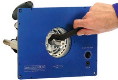
Fig. 16 View of OFL1.0 from above without reducing ring
