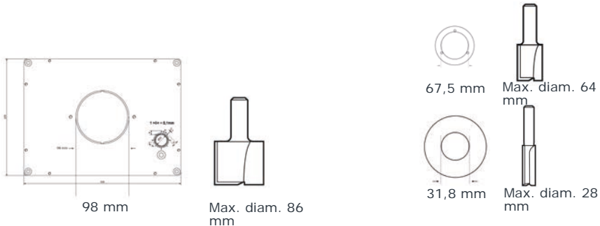
Fig. 17 Dimensions for bit selection
